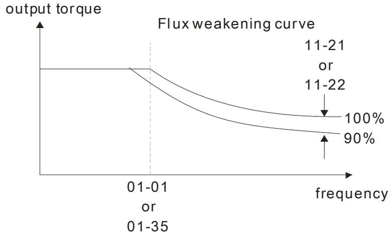
↖ **11-23** Speed Response of Flux Weakening Area Factory Setting: 65
