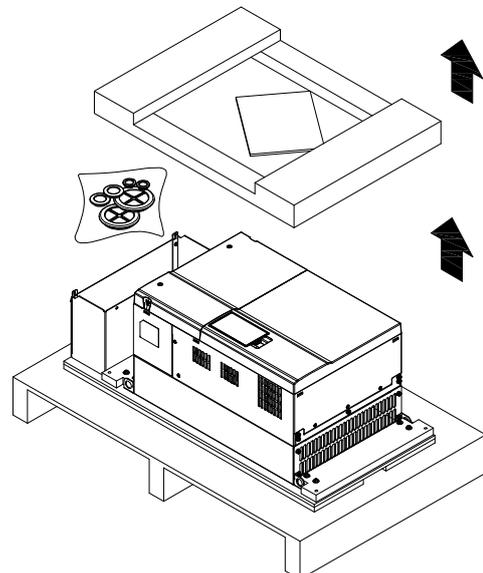
Lift the drive by hooking the lifting hole. It is now ready for installation.
