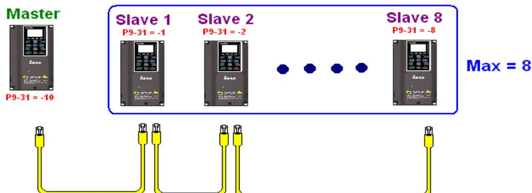
Master programming: In a program, D1110 can be used to define a slave station to be controlled (1-8, if set as 0, can jump between 8 stations). Afterwards, M1035 is set as 1, and the memory positions of the master and slave stations will correspond. At this time, it is only necessary to send commands to the correlation slave station address to control that station. The following is a register table connected with internal communications:
