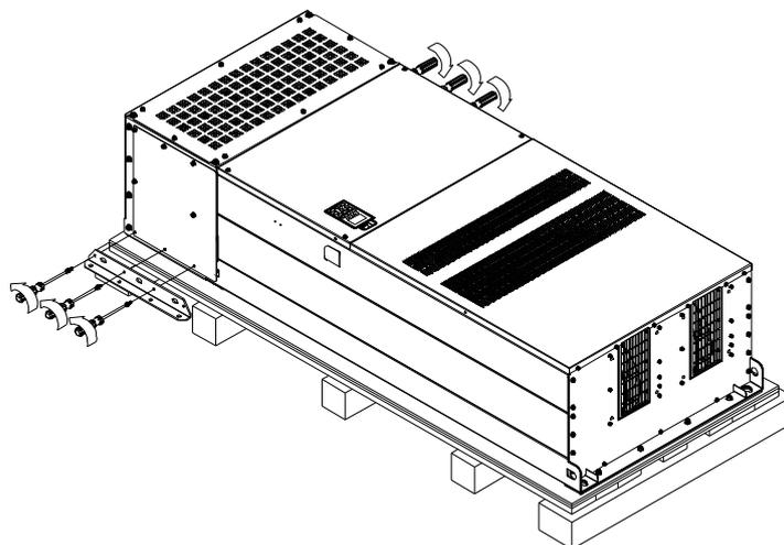
**Secure the drive from the internal.**
