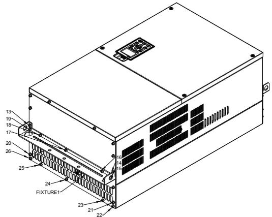
5. Place 4 of the M12 screws through Fixture 1&2 and plate then fasten the screws.
