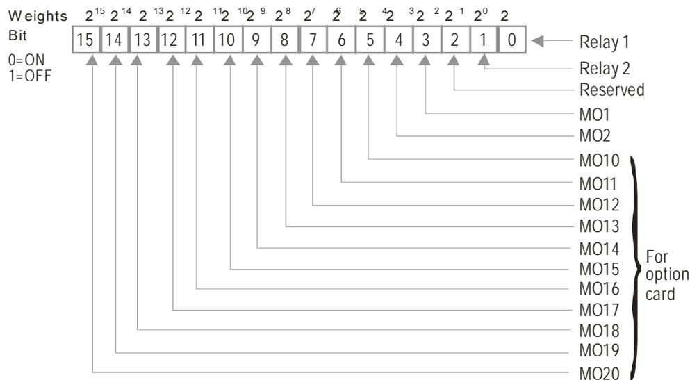
**02-52** Display External Output terminal occupied by PLC
