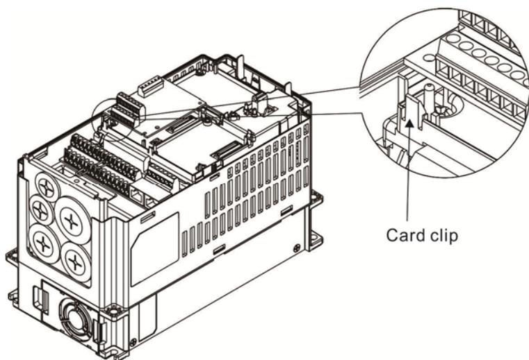
Twist to open the other card clip to remove the PCB.
