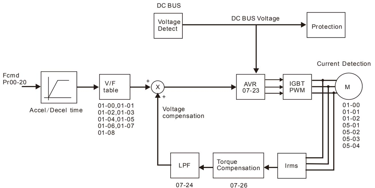
When 00-10=0, and set Pr.00-11 to 1, the V/F control + encoder diagram is shown as follows.
