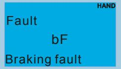
Fault<br>bF<br>Braking fault       | Brake resistor fault                                                                                                                                                                                                                                                          | If the fault code is still displayed on the keypad after pressing "RESET" key, please return to the factory.                                                                            |
