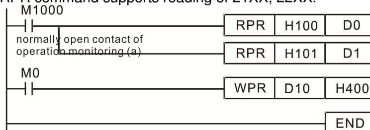
**Recommendation** Take care when using the WPR command. When writing parameters, because most parameters are recorded as they are written, these parameters may only be revised 109 times; a memory write error may occur if parameters are written more than 10<sup>9</sup> times.
