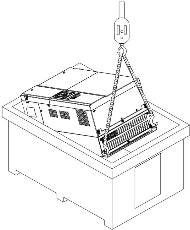
Loosen the 10 screws on the pallet, remove the wooden plate.
