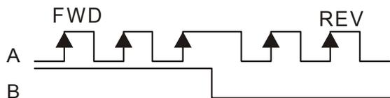
4: Phase A is a pulse input and phase B is a direction input. (L=forward direction, H=reverse direction)
