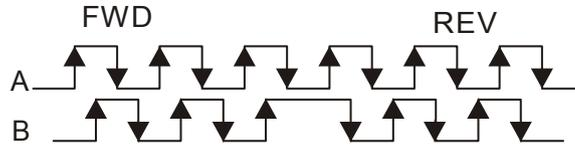
2: Phase B leads in a forward run command and phase A leads in a reverse run command
