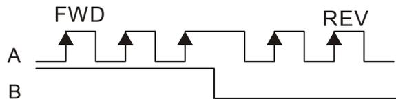
4: Phase A is a pulse input and phase B is a direction input. (L=forward direction, H=reverse direction)
