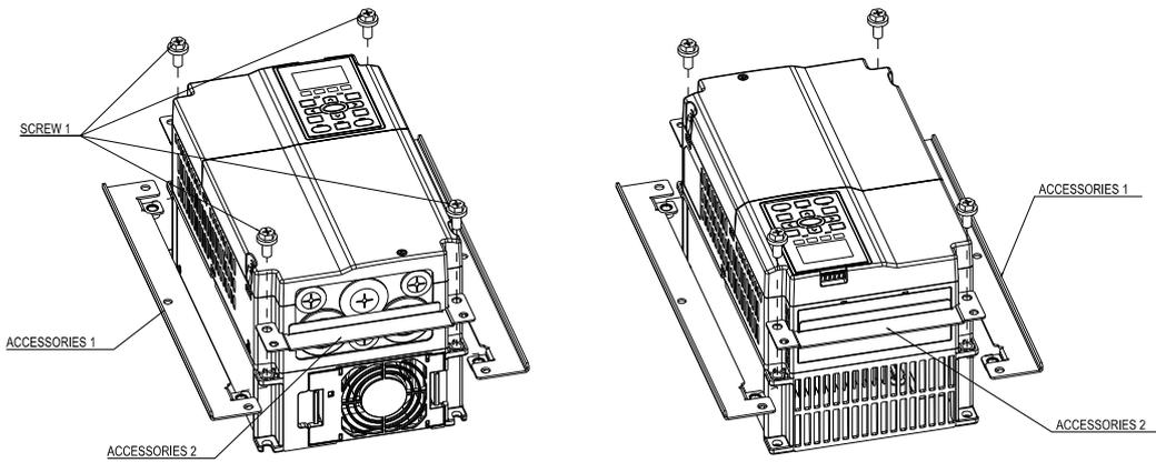
2. Plate installation, place 6 of the screw 2 (M6) through accessory 1&2 and the plate then fasten the screws. Screw torque: 25~30kg-cm (21.7~26lb-in). (As shown in the following figure)
