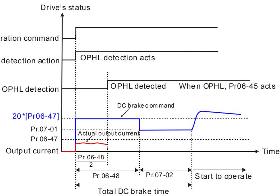
📖 Status 4: Motor drive is in stop; Pr06-48 ≠ 0 ; Pr07-02=0
