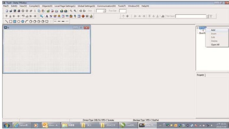
2. On the bottom right-hand corner of the HMI, click on a page number to edit or go to VIEW >HMI page to start editing main page. As shown in the image, the following objects are available. From left to right: Static Text, ASCII Display, Static Bitmap, Scale, Bar Graph, Button, Clock Display, Multi-state bit map, Units, Numeric Input and 11 geometric bitmaps and lines of different width. The application of Static Text, Static Bitmap, and geometric bitmap is the same as the editing startup page.
