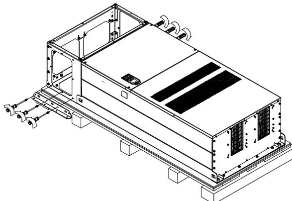
**Secure the drive from the external.** (Skip to the next step if this situation does not apply to you.) Loosen 8 of M8 screws on the both sides and place the 2 plates that were removed from the last step. Fix the plates to AC motor drive by fasten 8 of the M8 screws. (As shown in below)
