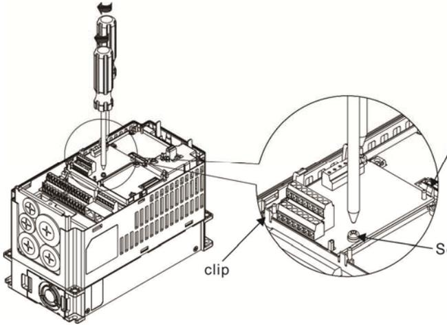
As shown in the figure on the left. Fasten, the screw after the PCB is clipped with the holes.
