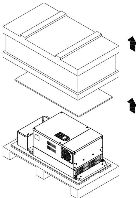
Loosen the 8 screws on the pallet as shown in the following figure.
