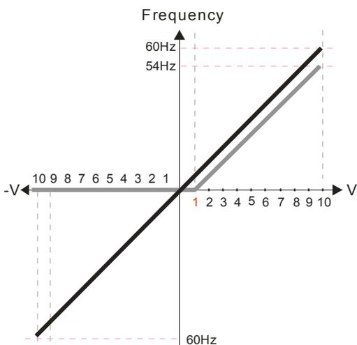
Pr.00-21=0 (Digital keypad control and d run in FWD direction)
