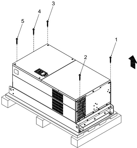
Loosen the 12 screws and remove the wooden plate.
