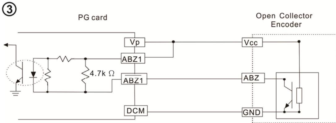
When wiring in this way, if there is a signal on EMC-PG010's A1, B1 and Z1, LED lights is OFF.
