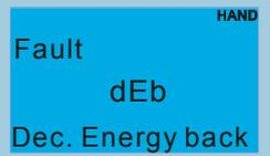
Fault<br>dEb<br>Dec. Energy back | When Pr.07-13 is not set to 0 and momentary power off or power cut, it will display dEb during accel./decel. stop.                                                                                                                                                            | <ol style="list-style-type: none"> <li>1. Set Pr.07-13 to 0</li> <li>2. Check if input power is stable</li> </ol>                                                                       |
