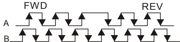
3: Phase A is a pulse input and phase B is a direction input. (L =reverse direction, H=forward direction)
