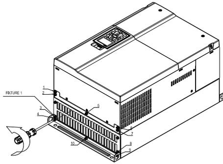
3. Fasten 4 screws (as shown in the following figure). Screw torque: 30~32kg-cm (26.0~27.8lb-in).
