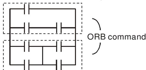
In the case of ANB and ORB operations, if a number of blocks are connected, they should be combined to form a block or network from the top down or from left to right.
