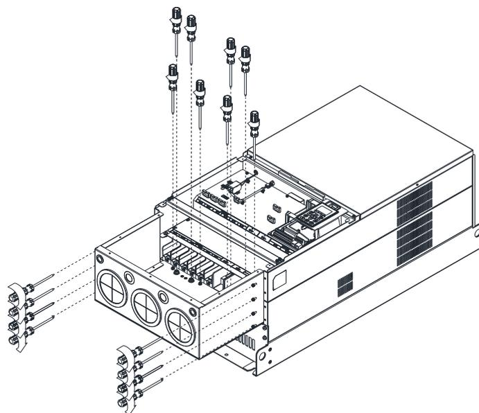
Fasten all the screws. Screw torque: 24~26kg-cm (20.8~22.6lb-in).
