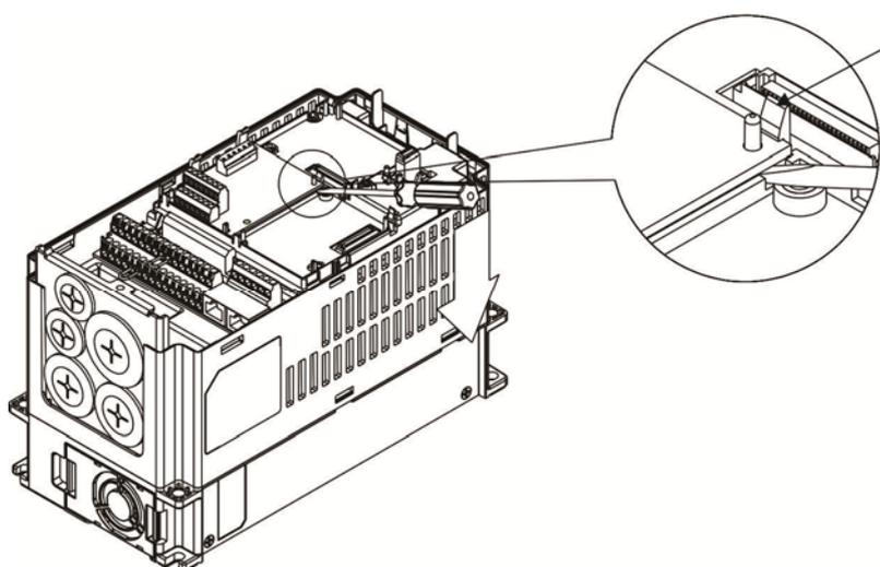
Twist to open the card clip. Insert a slot type screwdriver into the hollow to prize the PCB off the card clip.
