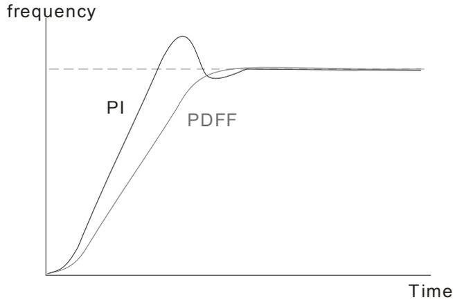
➤ **11-14** Low-pass Filter Time of ASR Output
