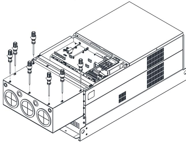
Place the cover back to the top and fasten the screws (as shown in the figure).
