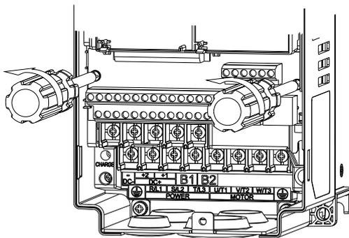
2. Remove the control board by pulling it out for a distance 6~8 cm (as 1 in the figure) then lift the control board upward (as 2 in the figure).
