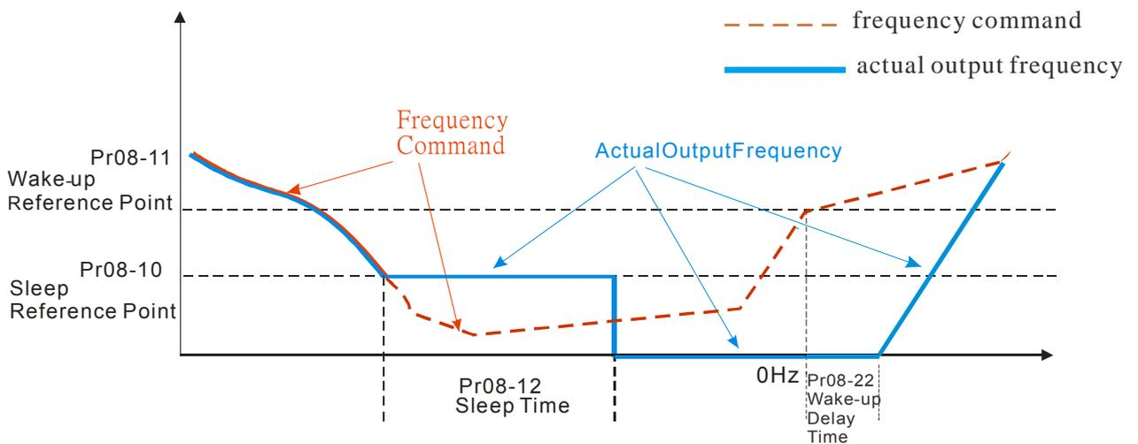
2) Frequency Command Calculation of the Internal PID
