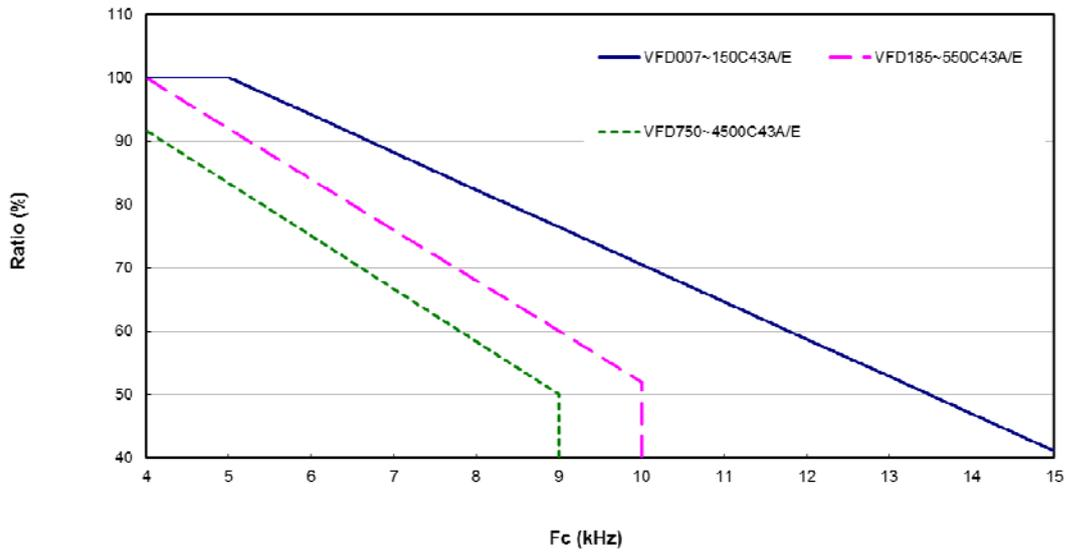
Derating Curve for Sensorless Control (230V, HD)
