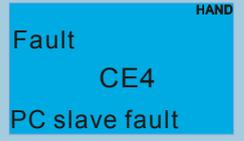
Fault<br>CE4<br>PC slave fault     | Data is written to read-only address                                                                                                                                                                                                                                          | Check if the communication address is correct                                                                                                                                           |
