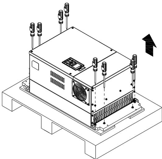
Loosen the 10 screws on the pallet and remove the wooden plate.
