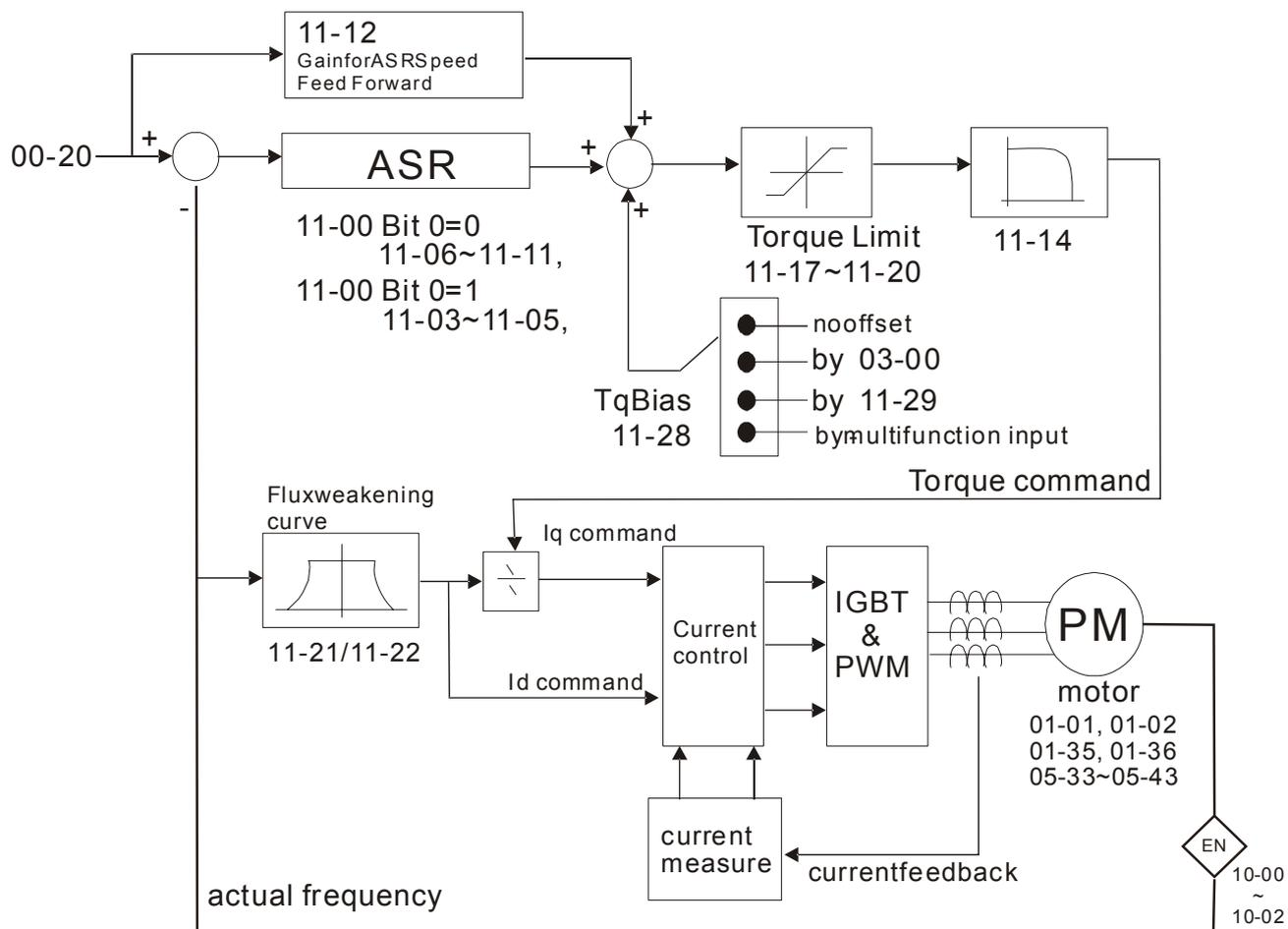
When 00-10=0, and set Pr.00-11 to 5, FOC sensorless (IM) control diagram is shown as follows.
