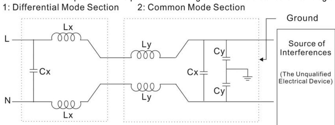
A filter is composed of a Differential Mode section (to eliminate noise below 150kHz) and a Common Mode section (to eliminate noise above 150kHz). For high-frequency noise, the inductor acts as a high impedance to form an open circuit and the capacitor acts as a low impedance to form a short circuit. Proper design and dimensioning of inductors and capacitors give a resonant circuit to absorb harmonic currents. Capacitor  $C_y$  is earthed to lead the harmonic currents to the ground.
