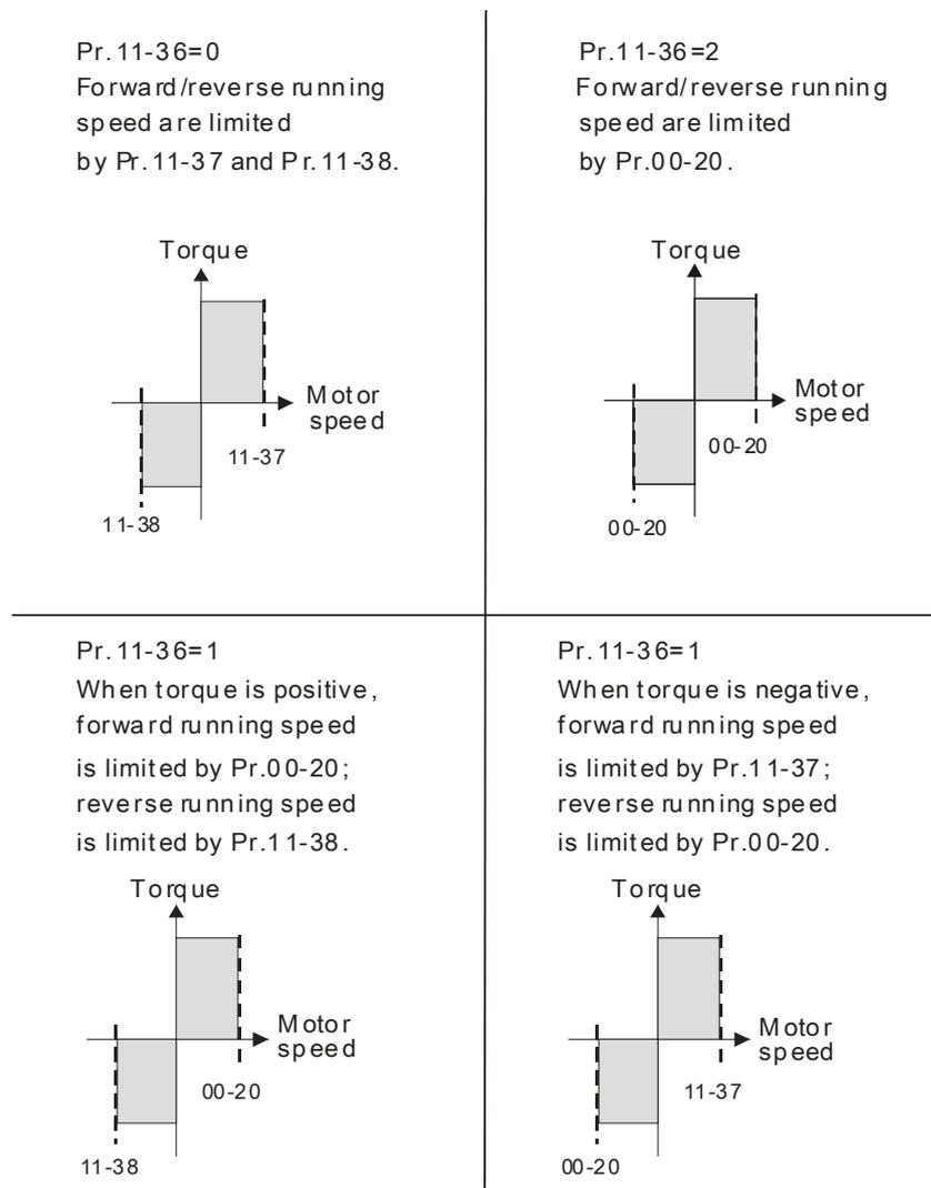
↗ **11-37** Forward Speed Limit (torque mode)
