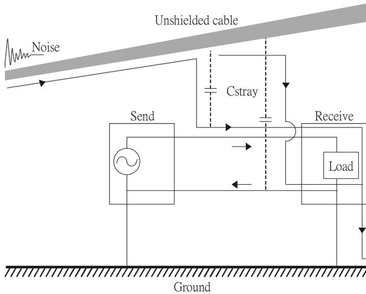
4. The common-mode noise of an unshielded power cable is transmitted to the ground via the stray capacitance. Since both shielded wire and unshielded wire are connected to a common ground, other systems can be interfered with by the common-mode noise that is transmitted from the ground back to the system via the shield. See Figure 4.
