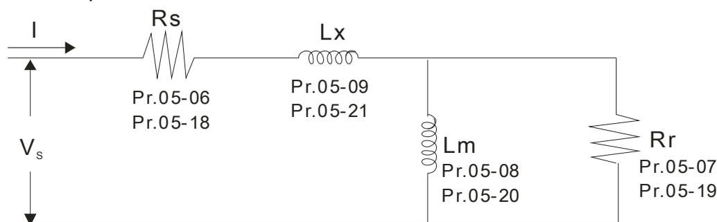
※ If Pr.05-00 is set to 2 (static test), user needs to input the no-load current value of motor into Pr.05-05 for motor 1/Pr.05-17 for motor 2.
