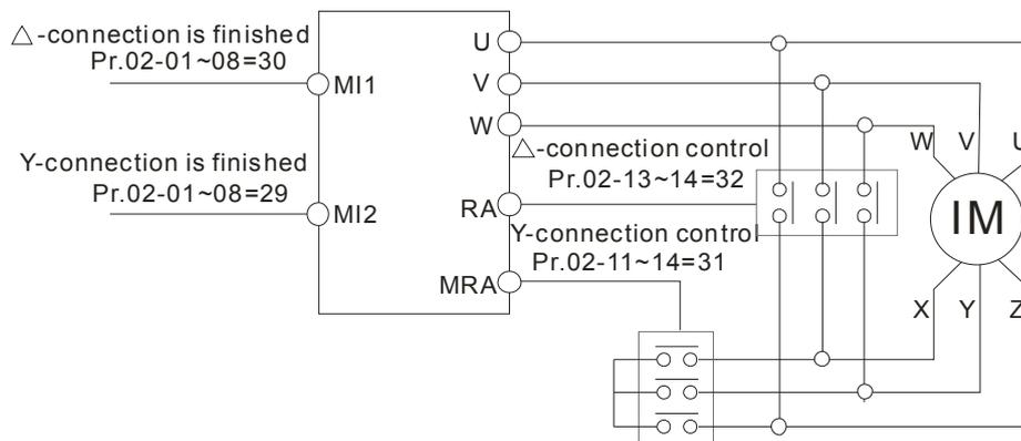
Y- $\Delta$  connection switch: can be used for wide range motor
