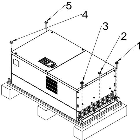
Loosen the 9 screws on the pallet and remove the wooden plate.
