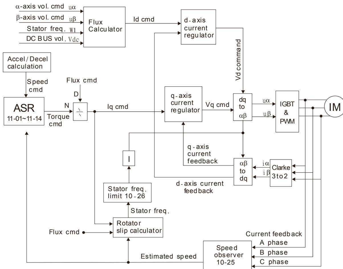
When 00-10=0, and set Pr.00-11 to 6, PM FOC sensorless control diagram is shown as follows:
