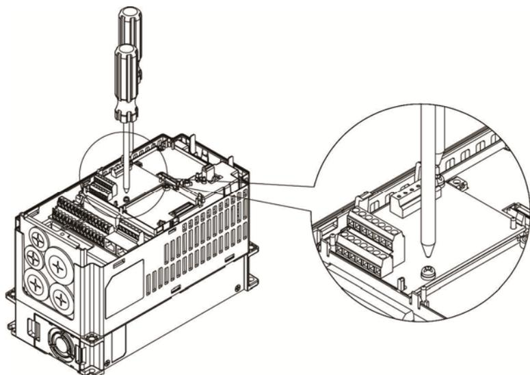
Remove the two screws as shown in the figure on the left.
