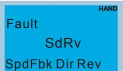
Fault<br>SdRv<br>SpdFbk Dir Rev  | Rotating direction is different from the commanding direction detected by the sensorless.<br>Solution<br>Verify if the parameter setting of the motor drive is correct<br>Increase the estimator's bandwidth and verify if parameters relating to the sensorless are correct. |                                                                                                                                                                                         |
