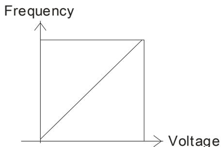
$$F_{\text{command}} = [(a_y \text{ bias}) * \text{gain}] * \frac{F_{\text{max}}(01-00)}{10\text{V or } 16\text{mA or } 20\text{mA}}$$
