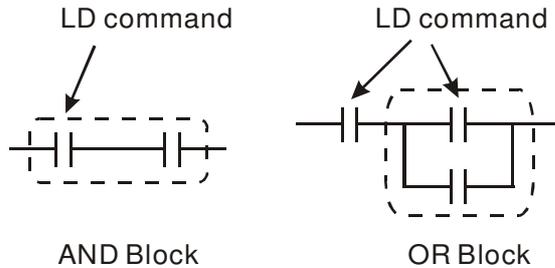
LDP and LDF have this command structure, but there are differences in their action state. LDP, LDF only act at the rising or falling edge of a conducting contact. (see figure below):
