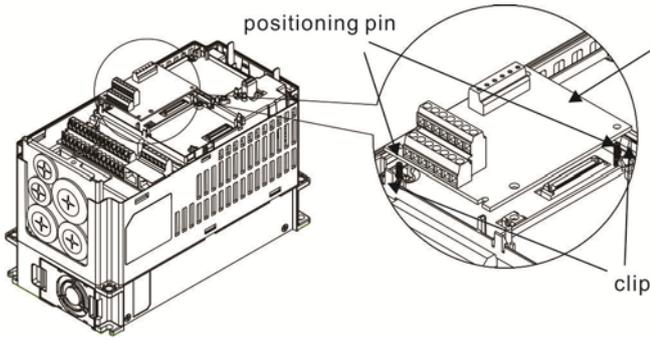
As shown in the figure on the left, aim the two holes at the positioning pin. Press the pin to clip the holes with the PCB.
