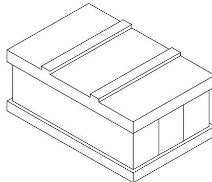
Loosen the 8 screws that fastened on the pallet and remove the wooden plate.
