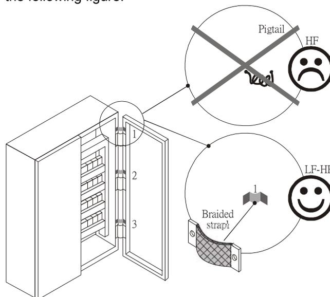
This is why a thick short ground wire must be implemented for connecting to the common grounding path or the ground busbar. Especially when a controller (e.g. PLC) is connected to an AC motor drive, it must be grounded by a short and thick conducting wire. It is suggested to use a flat braided conductor (ex: metal mesh) with a lower impedance at high frequencies.
