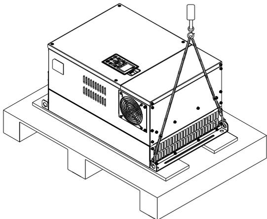
Lift the drive by hooking the lifting hole. It is now ready for installation.
