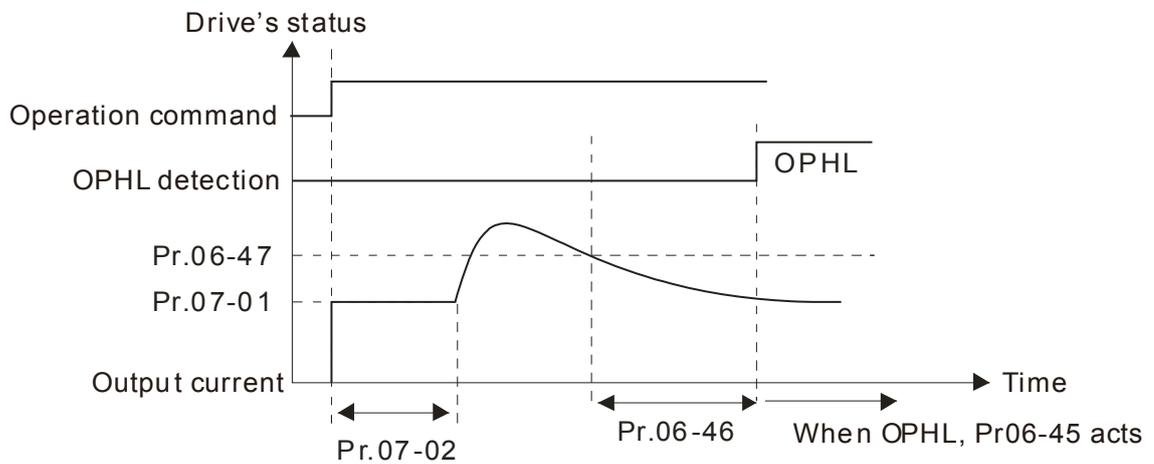
**Status 3: Motor drive is in stop; Pr06-48 ≠ 0 ; Pr07-02 ≠ 0**
