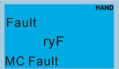
Fault<br>ryF<br>MC Fault         | Electric valve switch error when executing Soft Start.<br>(This warning is for frame E and higher frame of AC drives)<br><br>Do not disconnect RST when drive is still operating.                                                                                             |                                                                                                                                                                                         |
