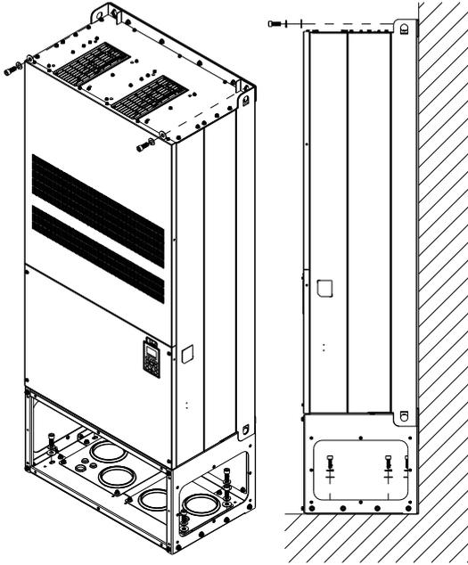
Secure the drive from the internal.
