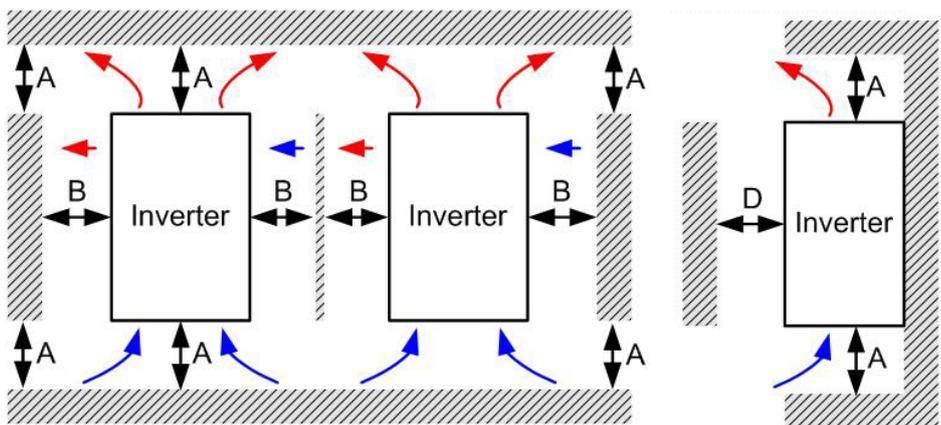
Multiple drives side-by-side vertical installation (Frame A~H)
