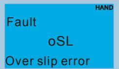
Fault<br>oSL<br>Over slip error  | It will be displayed when slip exceeds Pr.05-26 setting and time exceeds Pr.05-27 setting.                                                                                                                                                                                    | <ol style="list-style-type: none"> <li>1. Check if motor parameter is correct (please decrease the load if overload)</li> <li>2. Check the settings of Pr.05-26 and Pr.05-27</li> </ol> |
