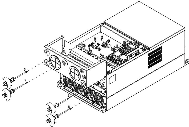
3. Install the conduit box by fasten all the screws shown in the following figure
