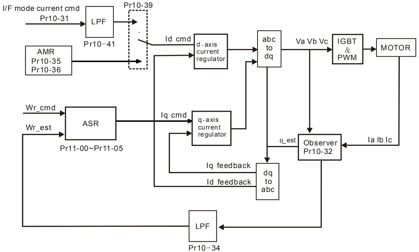
When 00-10=0, and set Pr.00-11 to 7, IPM FOC sensorless control diagram is shown as follows:
