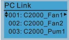
Use Up/Down key to select a parameter group to upload to VFDSOft. Press ENTER
