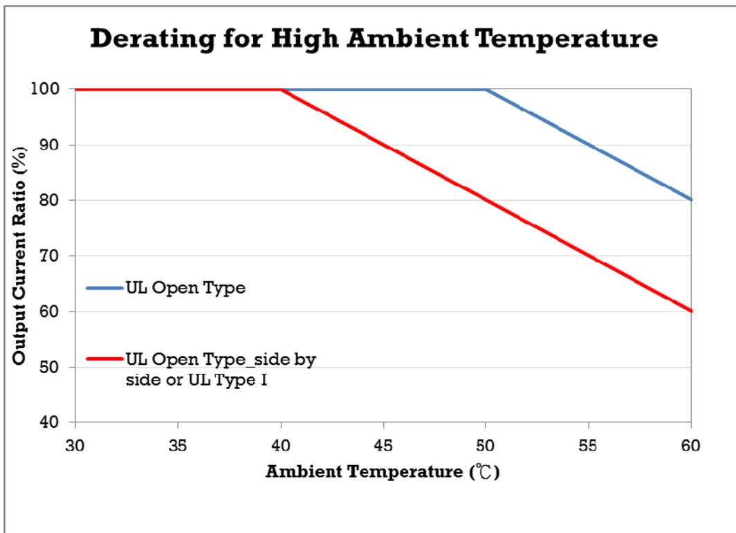
Advanced Control Derating Curve (Pr00-10=1, and Pr00-11=4~7; or Pr00-10=3, and Pr00-13=1~3)
