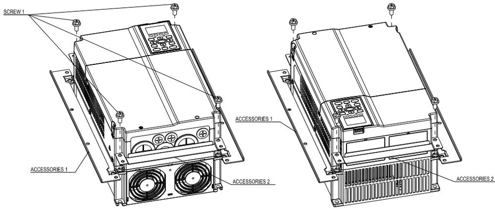
2. Plate installation, place 8 of the screw 2 (M6) through Accessory 1&2 and the plate then fasten the screws. Screw torque: 25~30kg-cm (21.7~26lb-in). (As shown in the following figure)
