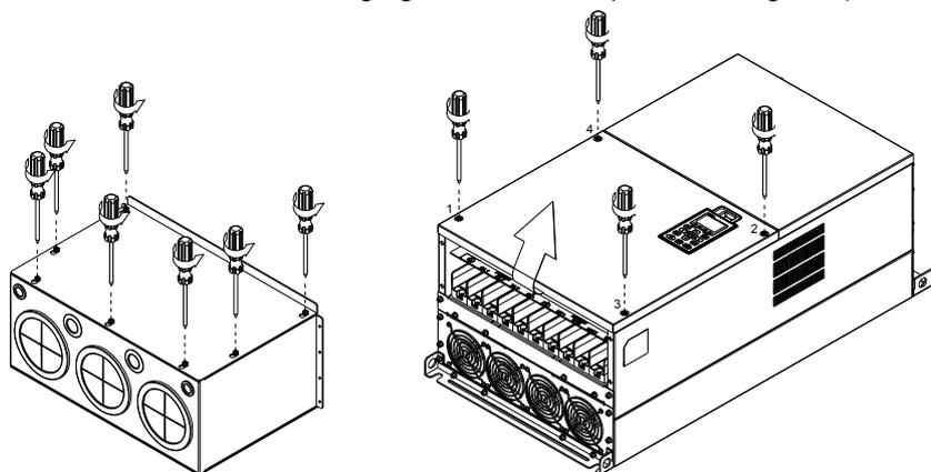
Remove the top cover and loosen the screws.
