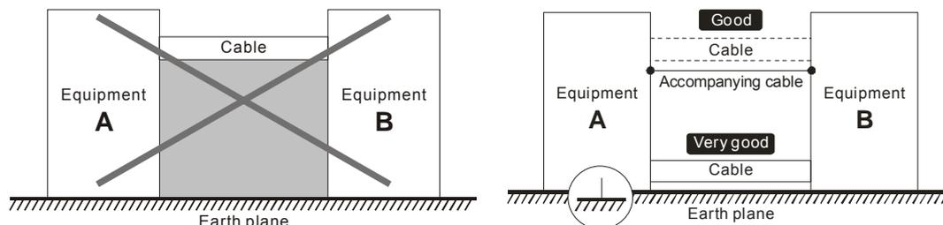
In order to avoid “Common Mode Noise”, please use parallel wires or twisted pair wiring. Follow this rule and also avoid long wires, it is suggested to place the two wires as close to each other as possible.
