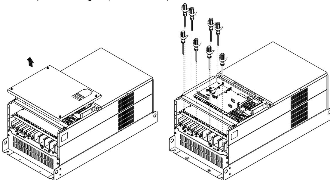
2. Install the conduit box by fastening all the screws shown in the following figure.
