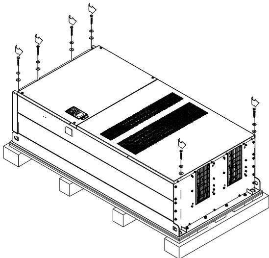
Loosen the 6 screws on the top then remove 6 metal washers and 6 plastic washers as shown in figure below.
