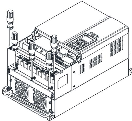
3. Install the conduit box by fasten the 5 screws shown in the following figure. Screw torque: 24~26kg-cm (20.8~22.6lb-in)
