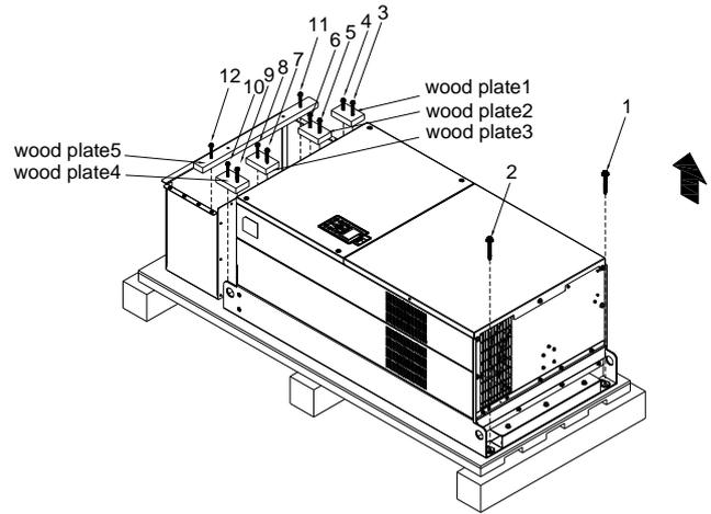
Lift the drive by hooking the lifting hole. It is now ready for installation.
