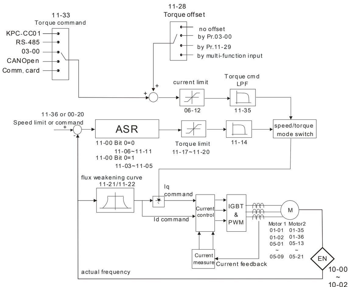
📖 TQC Sensorless (Pr00-13=2) control diagram is shown in the following:
