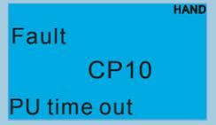
Fault<br>CP10<br>PU time out       | Keypad transmission time-out                                                                                                                                                                                                                                                  |                                                                                                                                                                                         |
