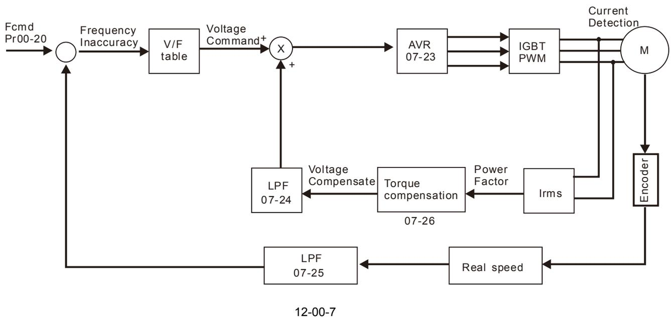
When 00-10=0, and set Pr.00-11 to 4, the PM FOCPG control diagram is shown as follows.
