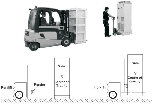
Note: High center of gravity, handle with care and avoid down. **2.3.2 Crane**
