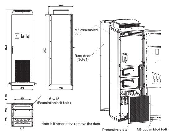
Install the equipment according to different ways. Open the front door, take down lower protective plate and, if necessary, remove the rear door. In particular, do not lose or damage the parts and fastening screws after removing the protective plate or the rear door. (Note: M12 expansion bolt is foundation bolt.) The installation diagram is shown as follows:
