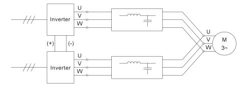
Wrong connection: The output cables meet at the inverter side or the cable from each phase of the inverter to the motor is in different length (as shown below).
