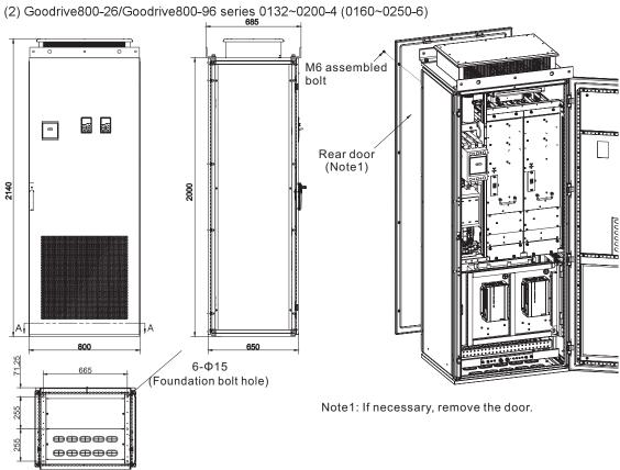
A-A Install the equipment according to different ways. Open the front door, then take down inner door component, and, if necessary, remove the rear door. In particular, do not lose or damage the parts and fastening screws after removing the protective plate or the rear door.
