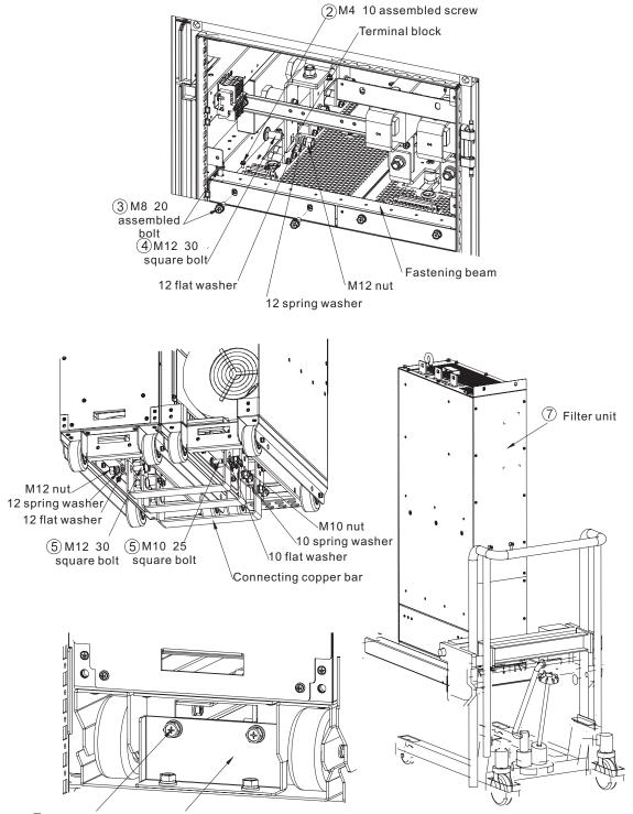
(6)M8 20 assembled bolt Lower fastener
