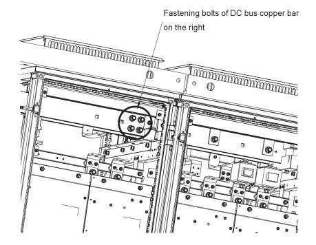
Install the removed fuses and copper bars at the original location after combining the bus copper bars
