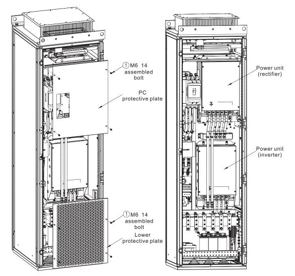
Note: The front door and inner door component are hidden in the figure.
