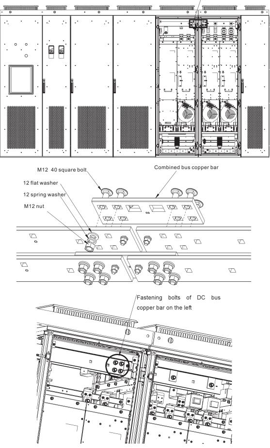
Mounting location of the combined bus copper bar (Front view)
