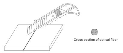
Requirement of optical fiber cutting: Use a utility knife to cut the optical fiber vertically, with one cut, and be sure to keep the cross section smooth and level without sharp angle or burr. Do not use diagonal pliers.
