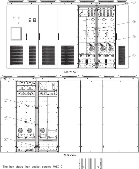
and spring washers 6 for combining cabinets are mounted as shown on the right.
