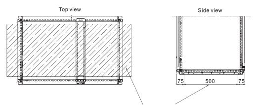
The space can be used for the layout of cable channel.
