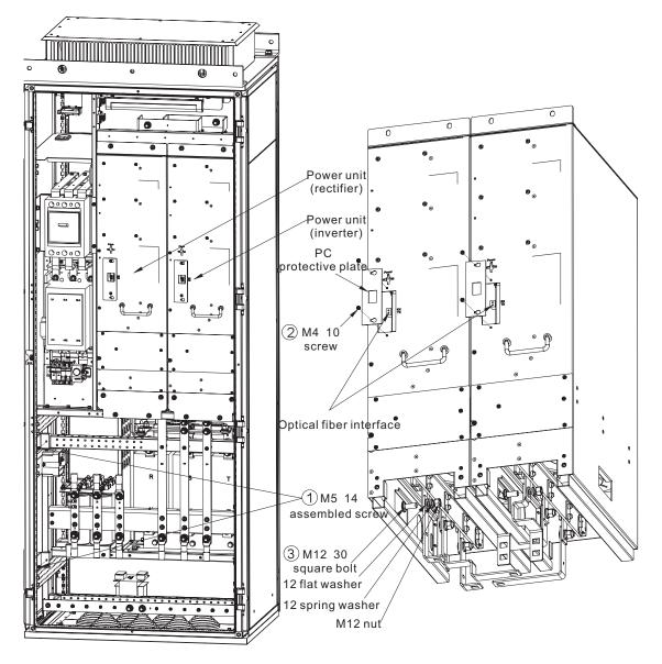
Note: The front door and inner door component are hidden in the figure.
