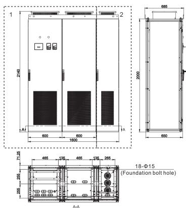
Install the equipment according to different ways. Open the front door, take down lower protective plate and, if necessary, remove the rear door. In particular, do not lose or damage the parts and fastening screws after removing the protective plate or the rear door. (Note: M12 expansion bolt is foundation bolt.)
