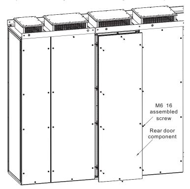
Step 3 Remove two power units at two sides of the combined cabinet and refer to (4) Maintenance for power unit (rectifier) in 3.4.1.3 for detailed information.
