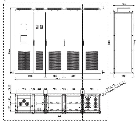
Install the equipment according to different ways. Open the front door, take down lower protective plate and, if necessary, remove the rear door. In particular, do not lose or damage the parts and fastening screws after removing the protective plate or the rear door. (Note: M12 expansion bolt is foundation bolt.)
