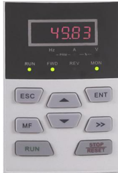
Fig. 4-6 Parameter setting status (b0-02 is set to 49.83Hz)
