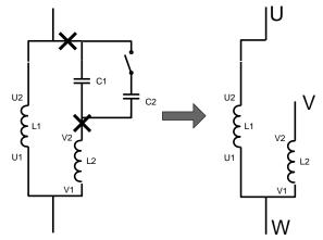
single-phase motor winding is as follows:
