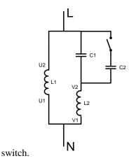
After removing the starting capacitor and the running capacitor, the internal wiring diagram of the
