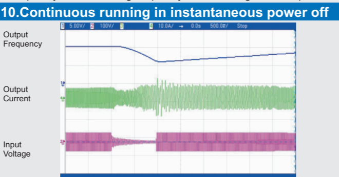
The inverter can keep running if the grid voltage drops and used in the situation with high requirement such as fiberic and textile production line.
