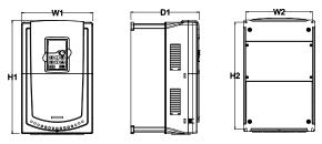
Wall installation of 500V 4-18.5kW VFDs
