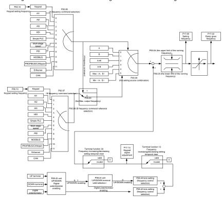
The VFDs support the shifting between different given channels, and the detailed shifting rules are as below:
