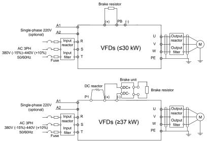
Figure 4-7 Main circuit connection diagram of 380V VFDs
