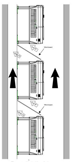
Figure 4-5 Vertical installation
