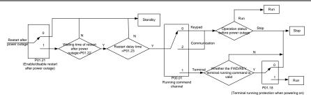
3. The starting logic figure of starting after the automatic fault reset.
