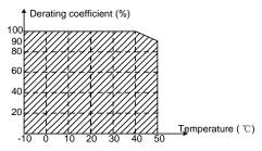
**Note:** It is not recommended to use the VFD at an environment with the temperature higher than 50°C. If you do, you shall be held accountable for the consequences caused.
