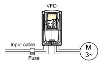
Figure 4-26 Fuse configuration
