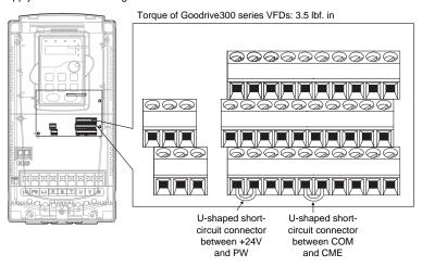
Figure 4-23 U-shaped short-circuit positions
