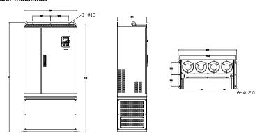
Floor installation of 380V 220-315kW VFDs
