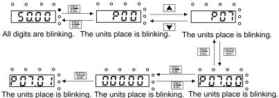
Note: When setting the value, you can press  $\rightarrow$  and  $\rightarrow$  +  $\checkmark$  to modify the value.
