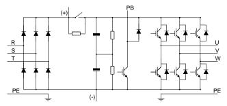
Figure 3-3 Main circuit of 500V VFDs (≤18.5kW)
