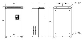
Wall installation of 660V 160-220kW VFDs
