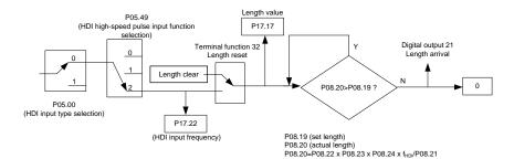
Note: The parameter of "Length arrival" is related to pulse output and the lasting time is 200ms.
