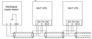
Above is "terminal" wiring diagram. Cable is a standard PROFIBUS cable consisting of a twisted pair and shielding layer. The shielded layer of PROFIBUS cable on all nodes is directly grounded. Users can choose the best grounding method according to the situation.
