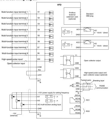
Figure 4-21 Control circuit wiring
