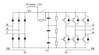
Figure 3-4 Main circuit of 500V VFDs (≥22kW)
