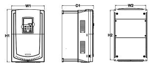
Wall installation of 380V 1.5-30kW VFDs
