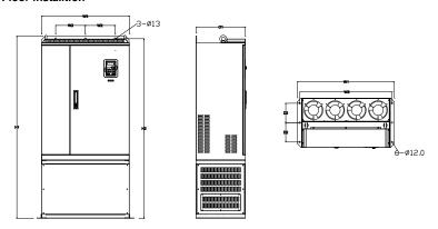
Floor installation of 660V 250-350kW VFDs
