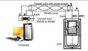
Figure 10-1 RS485 physical connection in single application
