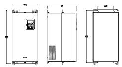
Wall installation of 500V 22-75kW VFDs
