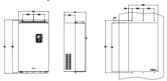
Flange installation of 660V 160-220kW VFDs
