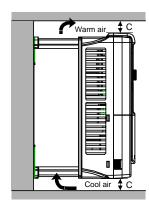
Figure 4-4 Parallel installation
