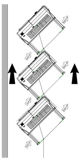
Figure 4-6 Tilt installation
