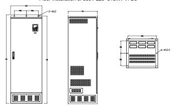
Floor installation of 380V 350-500kW VFDs
