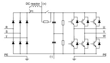
Figure 3-2 Main circuit of 380V VFDs (≥37kW)
