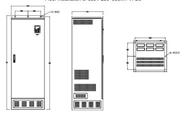
Floor installation of 660V 400-630kW VFDs
