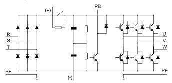
Figure 3-1 Main circuit of 380V VFDs (≤ 30kW)
