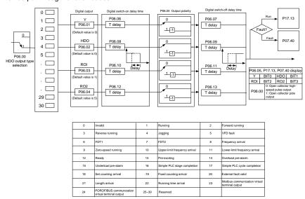
The following table is the option of the four function parameters and selecting the repeated output terminal function is allowed.
