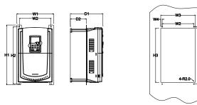
Flange installation of 380V 1.5-30kW VFDs
