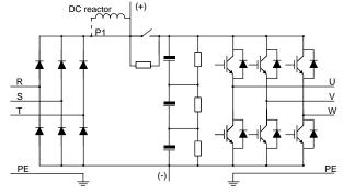
Figure 3-5 Main circuit of 660V VFDs
