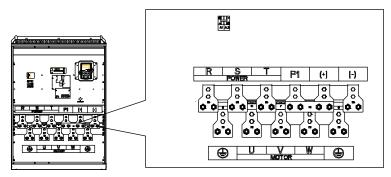
Figure 4-18 Main circuit terminals diagram of VFDs of 380V (220-315kW) and 660V (250-350kW)
