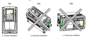
Figure 4-1 Installation direction of the VFD
