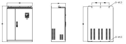
Wall installation of 660V 250-350kW VFDs
