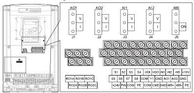
Figure 4-22 Control circuit terminals
