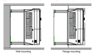
Figure 4-2 Installation mode
