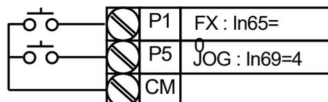
The jog operation is the second highest priority operation, after the dwell operation. If a jog operation is requested while operating the multi-step, up-down, or 3-wire operation modes, the jog operation overrides all other operation modes. The diagram above shows the example when the multi-function input is set to the NPN mode.
