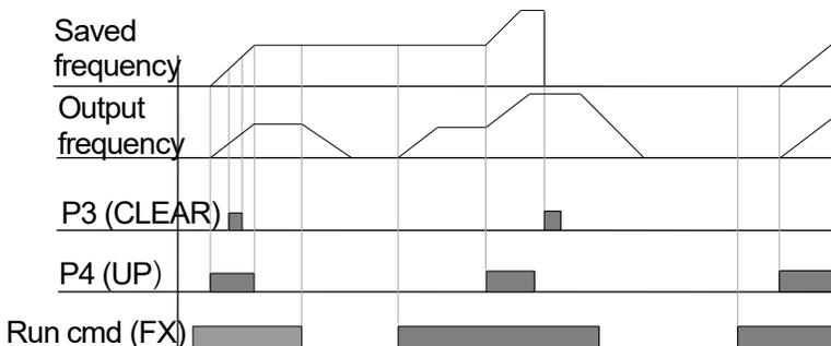
When the Ad66 code is set to 1: The motor accelerates by as much as the step frequency set by the Ad67 code at the multi-function input's positive edge that has been set as the Up terminal signal. The motor decelerates by as much as the step frequency set at the Ad67
