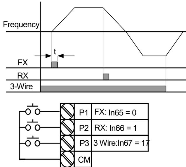
The 3-wire operation latches the signal input (the signal stays on after the button is released) as shown in the diagram above, and is used when operating the inverter with a push button switch.
