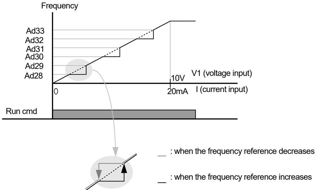
Use frequency jump to prevent motor operation at mechanical resonance frequencies. When jumping through a frequency bands while a motor accelerates and decelerates, operation frequencies cannot be set within the preset frequency jump band and the inverter operates at a constant speed.
