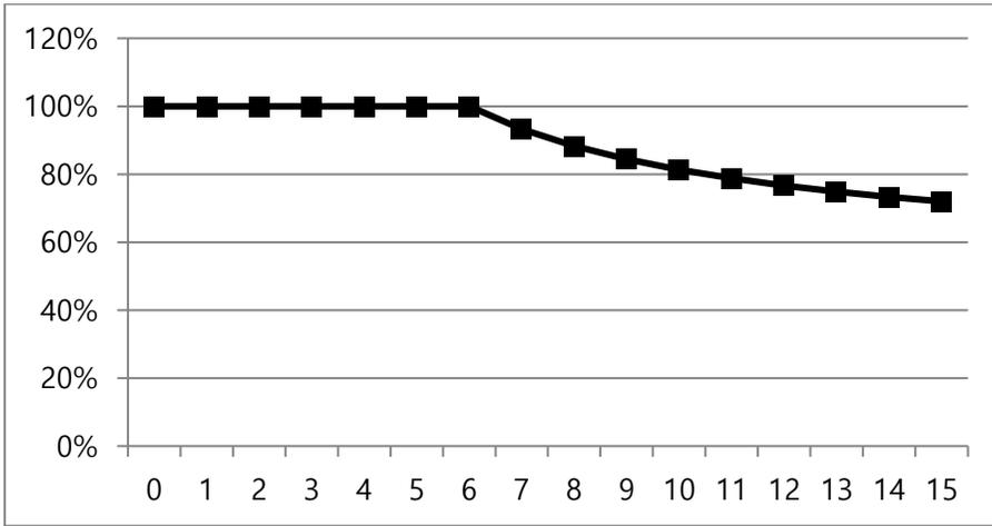
If the ambient temperature is high, and if the maximum carrier frequency for continuous full load conditions (4 kHz for A Frame 0.1 kW-1/0.2 kW-1 products, 6 kHz for B/C Frame 0.4 kW-1 – 2.2 kW-1 products) is exceeded, a protective feature may be activated to limit the carrier frequency (to 4 kHz / 6 kHz) to prevent damages to the product.
