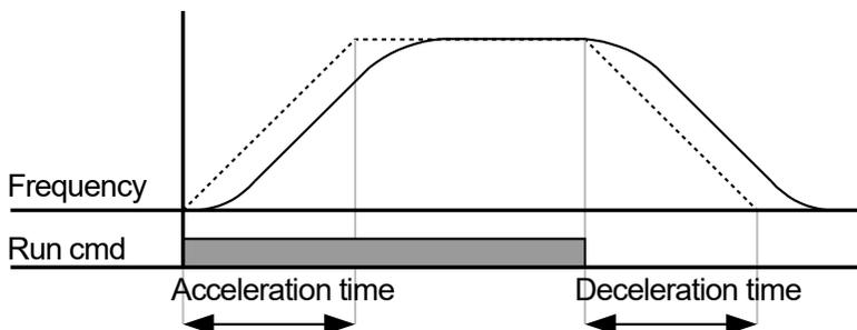
Ad03 defines the S-curve gradient level as a percentage, up to half of the total acceleration and deceleration (Acc Start and Dec Start) values. You can set the Ad03 parameter to a
