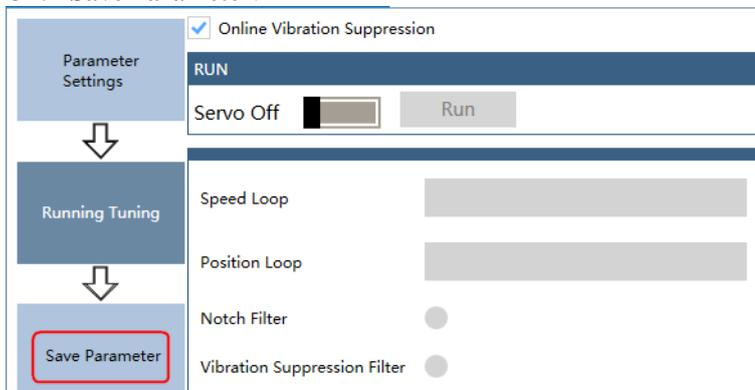
Step 14 Check the **RESULT**, and click **Save**, the settings of parameters will be written into the Drive automatically.
