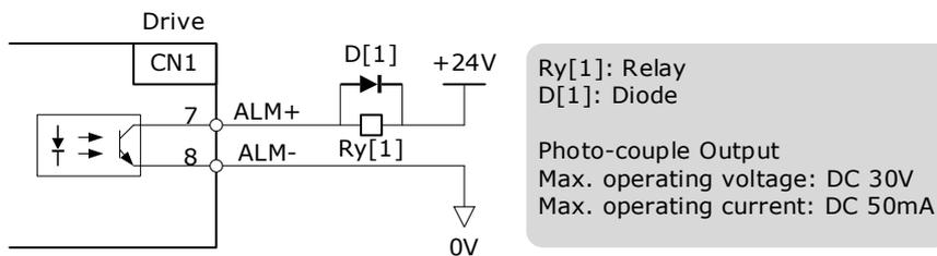
An external +24V I/O power supply is required.
