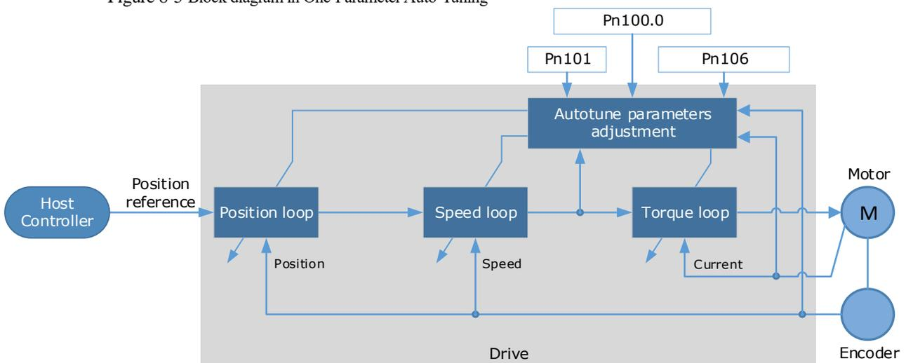
Before performing One-Parameter Auto-Tuning, you need to manually set the following parameters:
