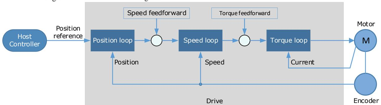
In general, the differential of the position reference is used as the feedforward, you can also set the feed forward by the controller or other application functions.
