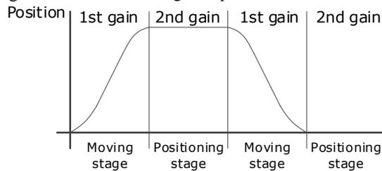
The parameters of the first gain and the second gain are as follows.
