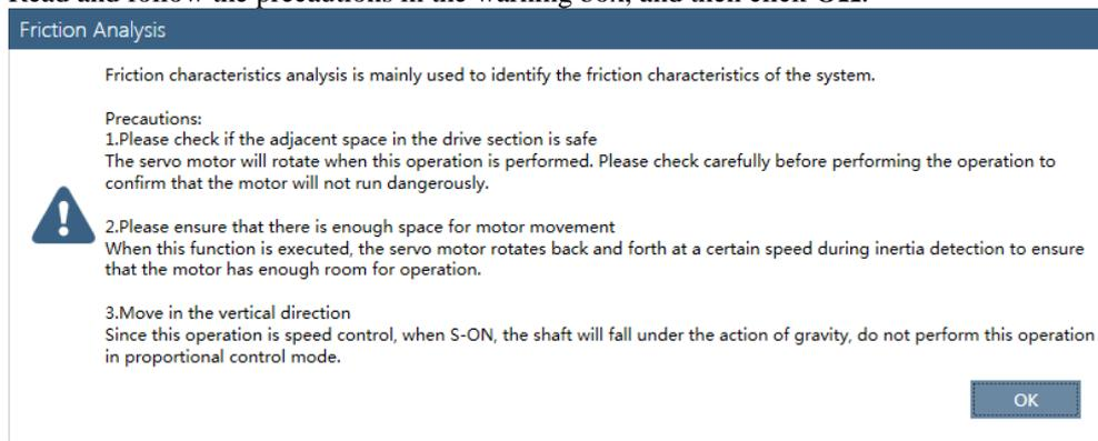
Step 3 The **Friction Analysis** window will be displayed in **Function Display Area**.
