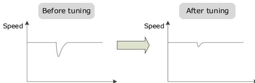
The load torque compensation function is to compensate the load torque compensation to the torque reference through the load torque observer.
