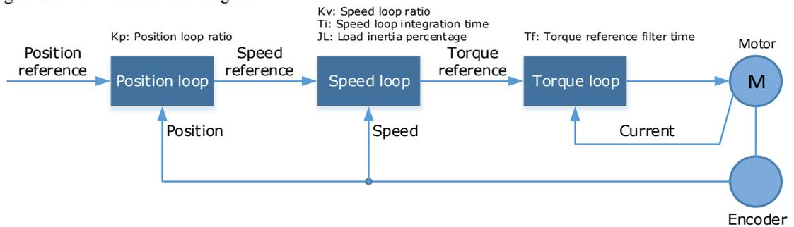
**NOTE:** only the basic tuning parameters during the tuning are shown in the figure.
