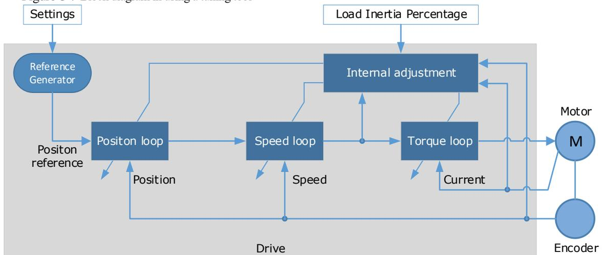
The reference generator plans an appropriate position reference according to the settings of relevant parameter.
