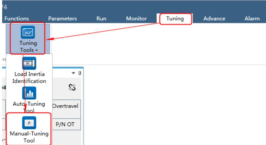
Step 2 The **Manual-Tuning Tool** window will be displayed in **Function Display Area**.
