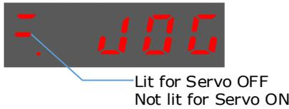
Step 4 Press [M] key to Servo ON (supply power to Motor).
