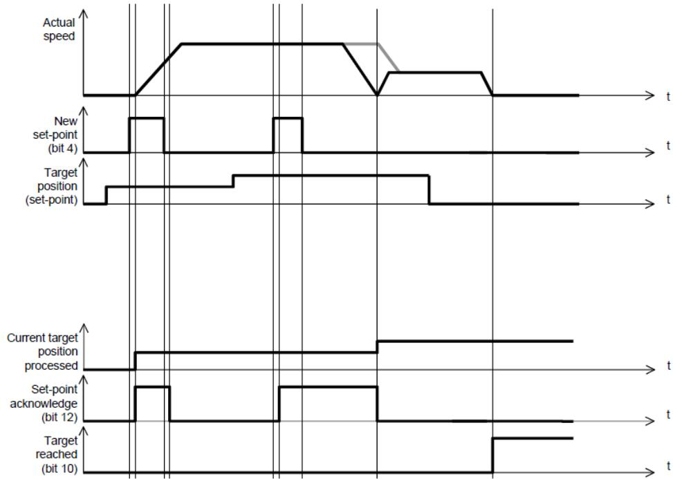
When the speed profile is S (motion\_profile\_type=2), only **Continuous-step setting** is available. 6083h (profile\_acceleration) limits max acceleration, and 6081h (profile\_velocity) limits max speed. 60A4-01 h (VAR Profile\_jerk1) limits the jerk. Only symmetrical S linear is available currently.
