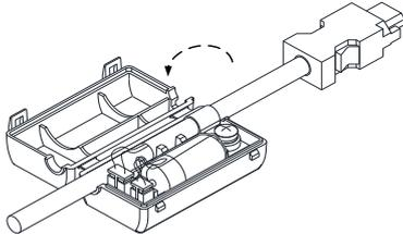
Step 3 Remove the old battery and mount a new battery.
