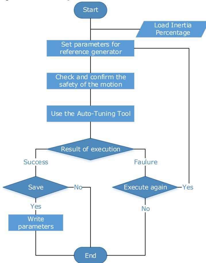
The following parameters are automatically adjusted when using the auto-tuning tool.
