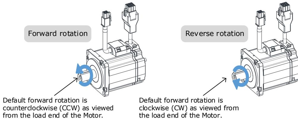
**NOTE:** The rotation direction of the Motor depends on the setting of Pn001.0 (CCW, CW). The figure above shows the default setting.
