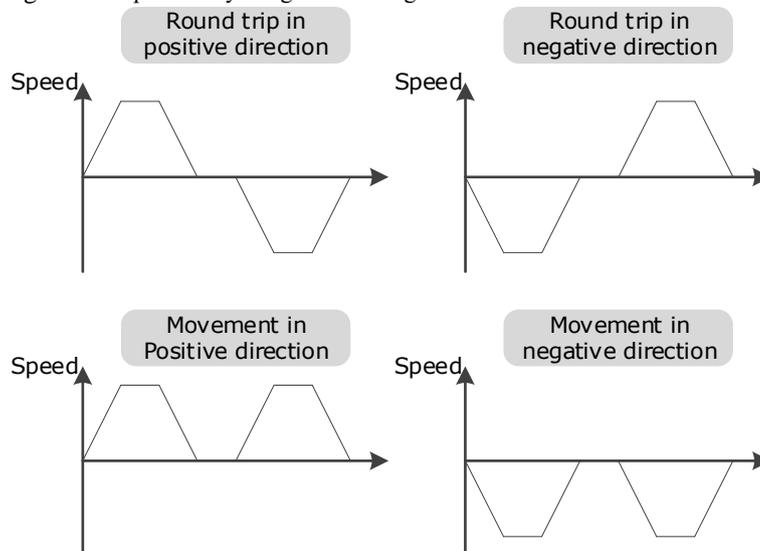
You shall set the Rotations (Pn164 and Pn168) and Max Speed (Pn165 and Pn169) to a proper value. If the Rotations is set too small or the Max Speed is set too large, it is possible that the maximum speed set cannot be reached. In this case, it is necessary to increase the Rotations or decrease the Max Speed.
