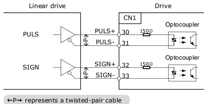
[Connection Example for Open-Collector Output]
