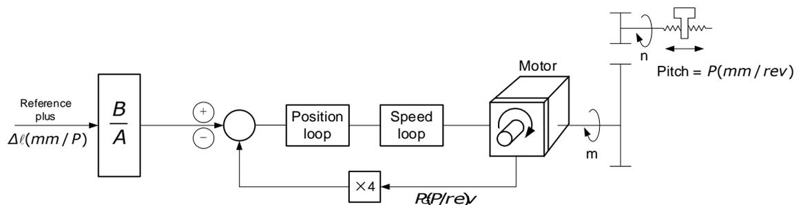
Where: Δl is the reference unit; P<sub>G</sub> is the encoder pulse; P is the pitch of the ball screw; m/n is the reduction ratio.
