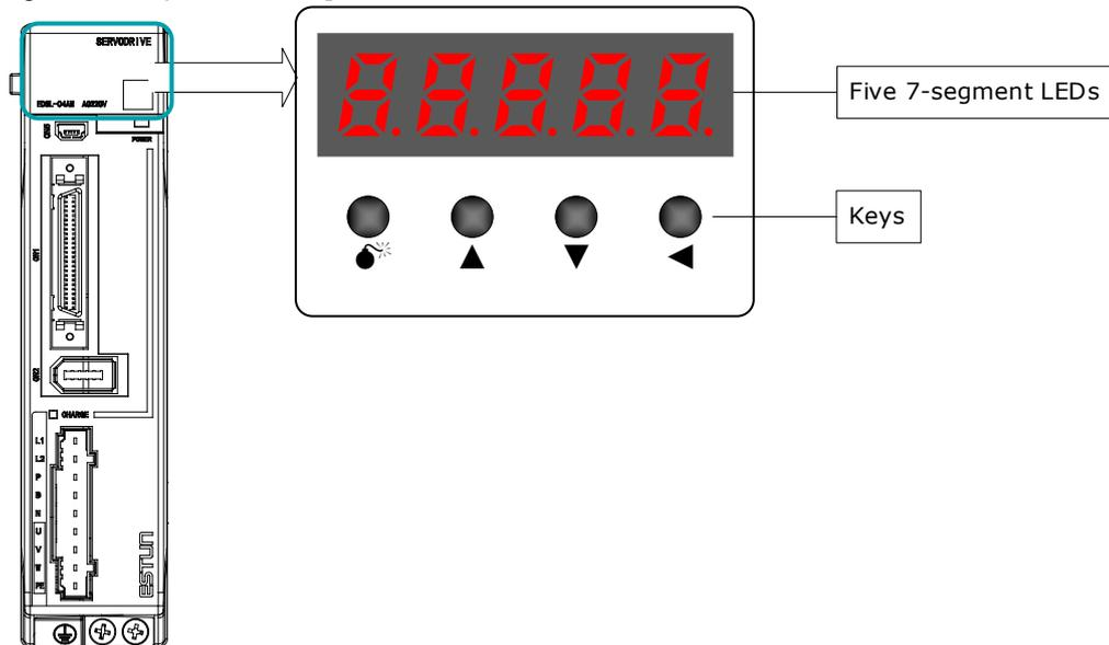
The names and functions of the keys on the Panel Operator are as follows.
