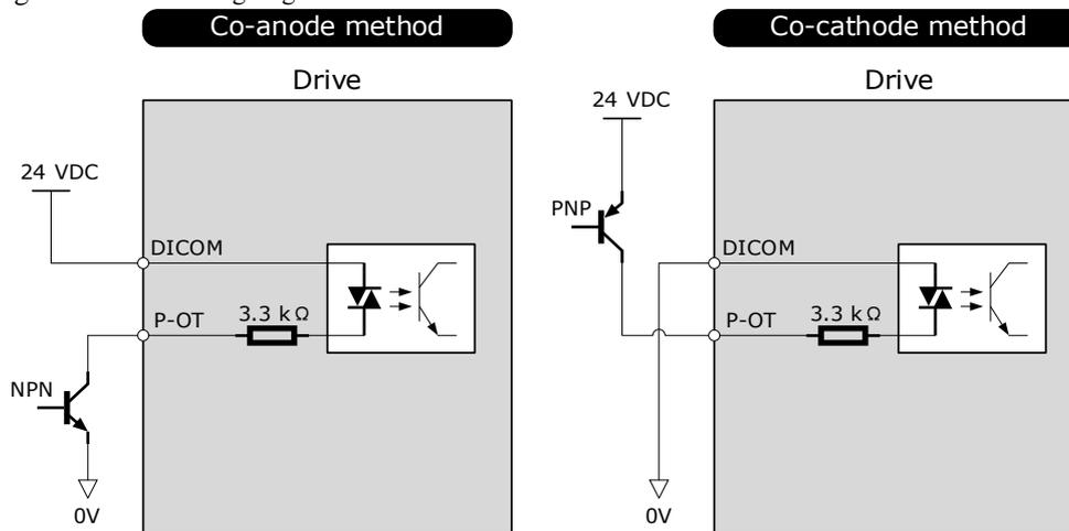
You can assign the input signals by Pn509 and Pn510. For the input signal allocation, see the section 5.7 IO Signal Allocation.
