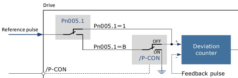
Inhibit (INHIBIT) is switched via /P-CON signal:
