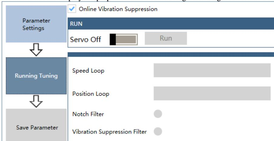
The setting will be written into the Drive automatically after you check or uncheck **Online Vibration Suppression** option.
