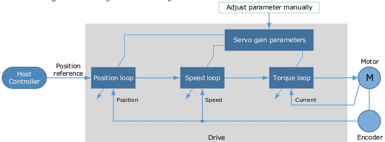
It is necessary to adjust the three-loop control parameters of the Servo from the inside out, that is, the adjustment sequence is **Torque loop** → **Speed loop** → **Position loop**. In addition, in order to meet the stability, the bandwidth setting should be the largest in the torque loop, the speed loop is the second, and the position loop is the smallest.
