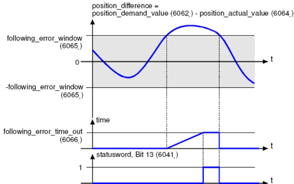
The deviation of the actual position value (`position_actual_value`) from the desired position value (`position_demand_value`) is named following error. As shown in figure above, if for a certain period of time this following error is bigger than specified in the following error window (`following_error_window`) bit 13 (`following_error`) of the object statusword will be set to 1.
