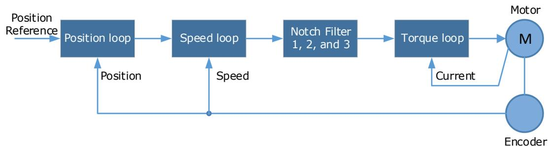
Figure 8-19 shows the relevant parameters for the notch filter. Since the notch filter can attenuate the signal at the notch frequency, if you set a proper frequency (Pn181, Pn184 or Pn187), depth (n182, Pn185 or Pn188) and width (n183, Pn186 or Pn189), the vibration signal in the torque reference can be filtered.
