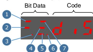
The display meaning of each segment on Bit Data are shown in Table 4-1, and they have different meanings under Speed or Torque Control Mode and Position Control Mode
