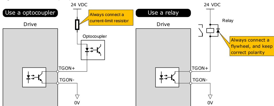
The maximum permissible voltage and current of the optocoupler output circuit inside the servo drive are as follows:
