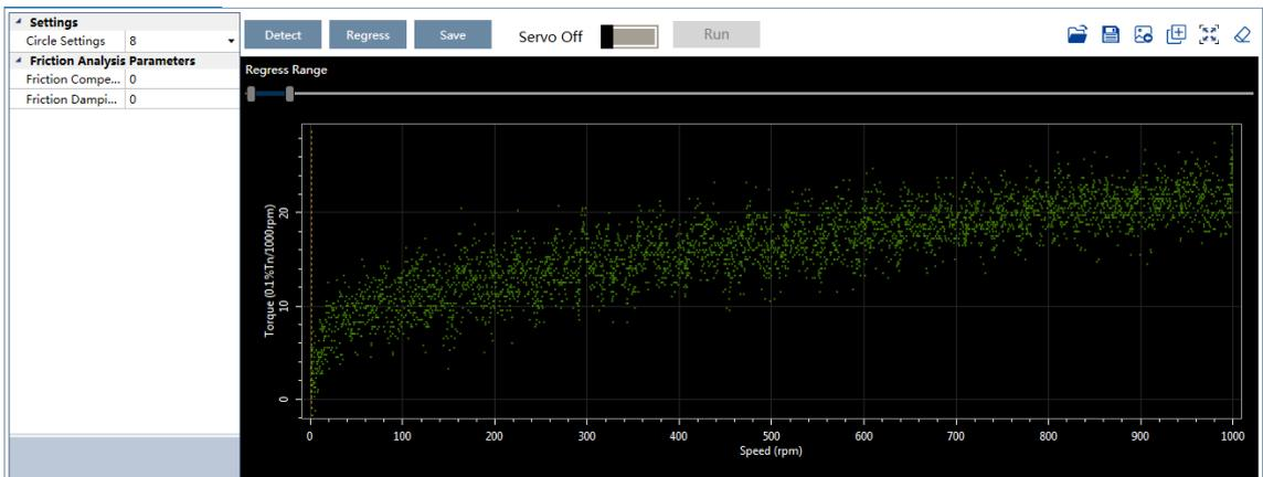
Step 9 Move **Regress Range** for setting a proper analysis range of Speed.
