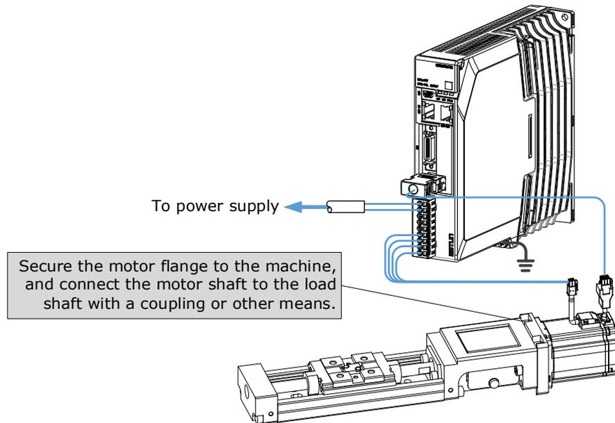
Step 5 Turn ON the power supplies to the machine and host controller and turn ON the control power supply and main circuit power supply to the Drive.
