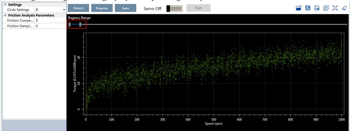
Step 10 Click **Regress** for calculating the **Friction Compensation Gain** and **Friction Damping Proportion**.
