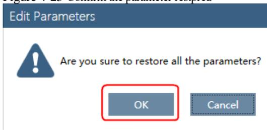
Step 3 ESView V4 will send the **Restore Parameters** command to the Drive, and then the Drive will execute the **Restore Parameters**.
