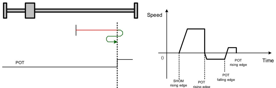
Homing modes 9 and 0, using deceleration point as overtravel switch, and origin as motor's Z signal
