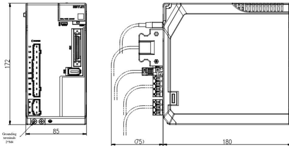
400VAC, rated power from 5kW to 7.5kW
