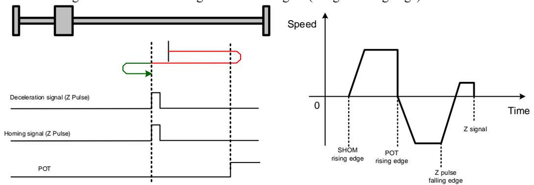
Homing modes 7 and 8, using deceleration point and origin as overtravel switch
