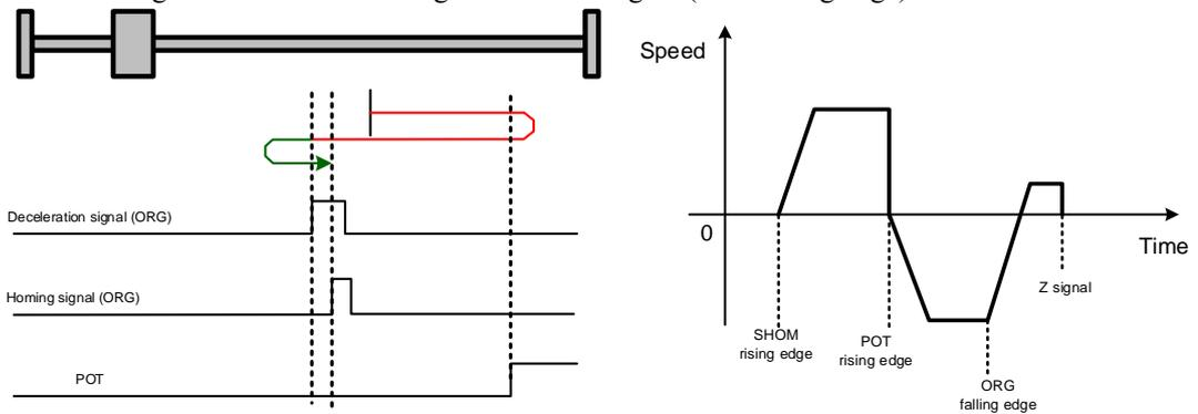
Homing modes 5 and 6, using origin as motor's Z signal
