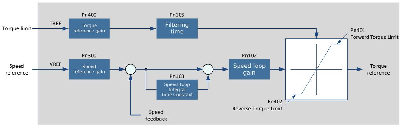
[Note] There is no issue with input voltage polarity of the analog voltage reference for torque limiting. The absolute values of both + and – voltages are input, and a torque limit value corresponding to that absolute value is applied in the forward or reverse direction.
