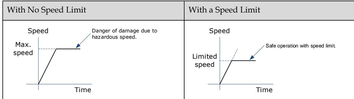
[Note] The actual limit of motor speed depends on the load conditions on the motor.
