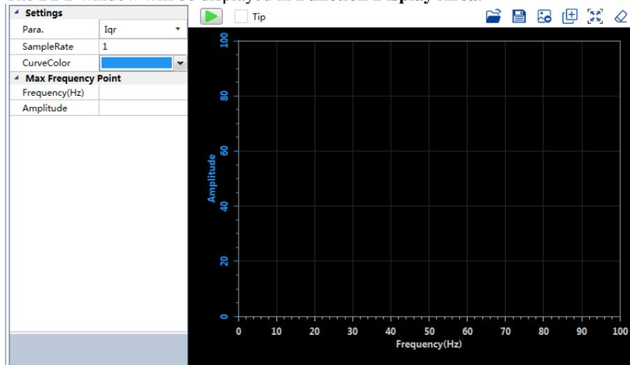
Step 3 Set the necessary parameters before performing the FFT function.
