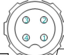
Recommended wire diameter for U, V, W and FG:1mm<sup>2</sup>
