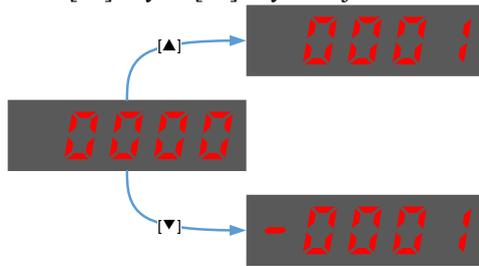
[Note] The adjustment range of the offset is -1024 to 1024.
