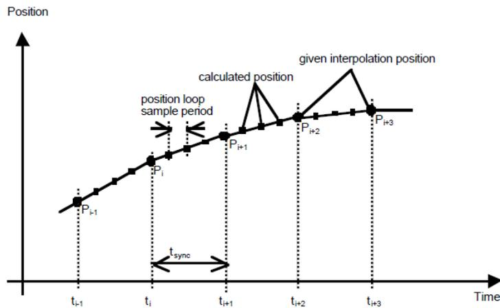
$P_i$ : interpolation position set by the host;  $t_{sync}$ : sync period
