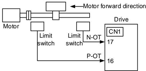
Using the overtravel function is not necessary for rotating applications such as rotary tables and conveyors. No wiring for overtravel input signals is required.
