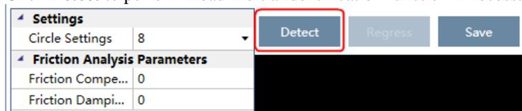
Step 5 Set **Circle Settings** for the Motor rotation when performing **Friction Analysis** function.
