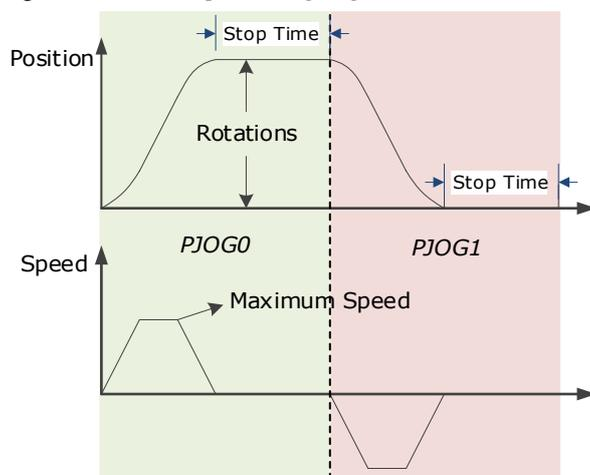
The Drive will operator the Motor repeatedly according to the parameter settings of the two operation patterns until you stop the program jogging operation manually.
