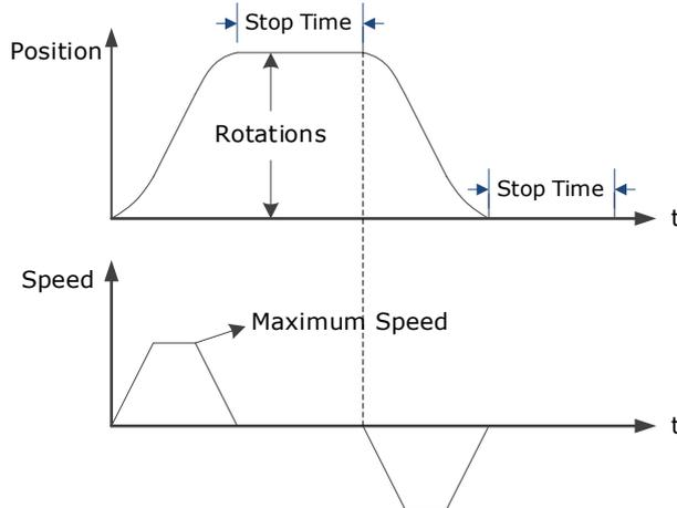
The Drive will operator the Motor repeatedly according to the parameter settings of the two operation patterns until the tuning is completed. You can set the parameters Pn164 and Pn168 to a negative value for reversing the Motor, so that there are four ways of the operation in the program jogging, as is shown in Figure 8-9.
